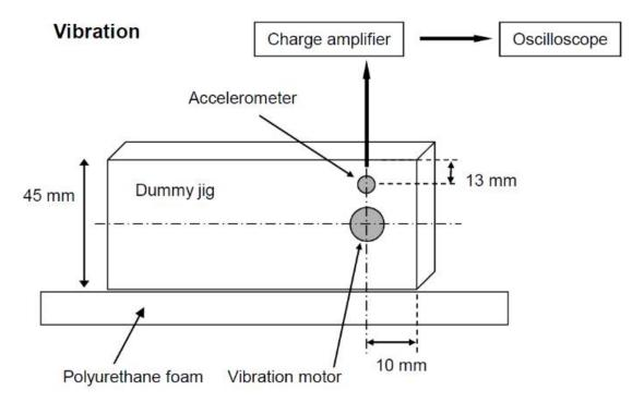
Specification of the dummy Jig
